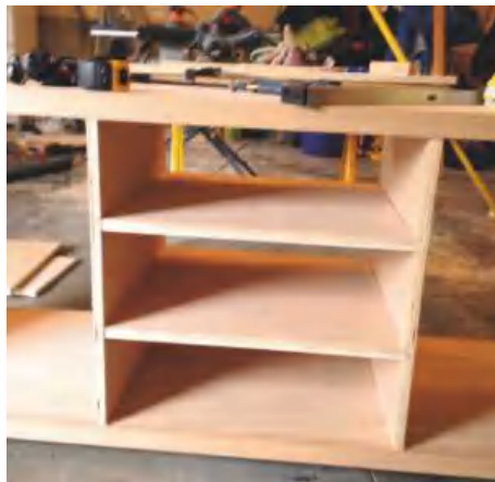
STEP 13. The next job is to measure the centre shelves and secure with pocket screws
